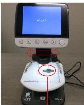
Put object on the stage, then adjust the height, then focus the camera.
