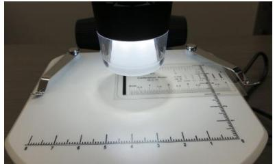
Remove the object and put the calibration scale on the stage.
