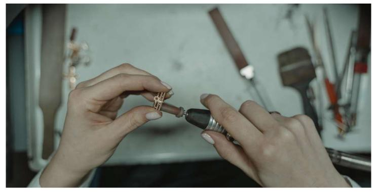
Micro grinder is a hand-held power tool used for cutting, sanding, carving, polishing, and several other applications.
