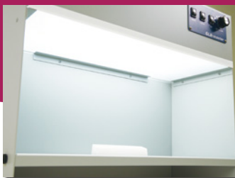
Special diffuser suitable for the grading is set under LED illumination.
