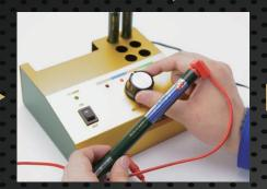
3. Touch the replating area with clamp or pin.
